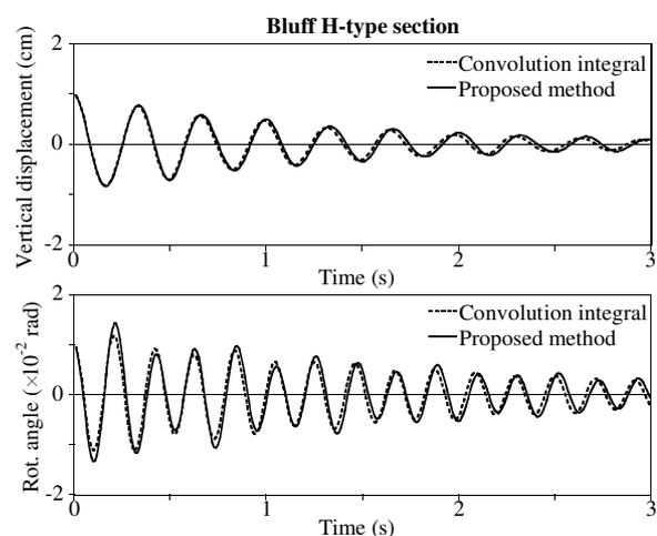
Fig. 4: Free vibration responses at the wind velocity of 8m/s for the bluff H-type section
