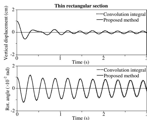
Fig. 2: Free vibration responses at the wind velocity of 15m/s for the thin rectangular section
