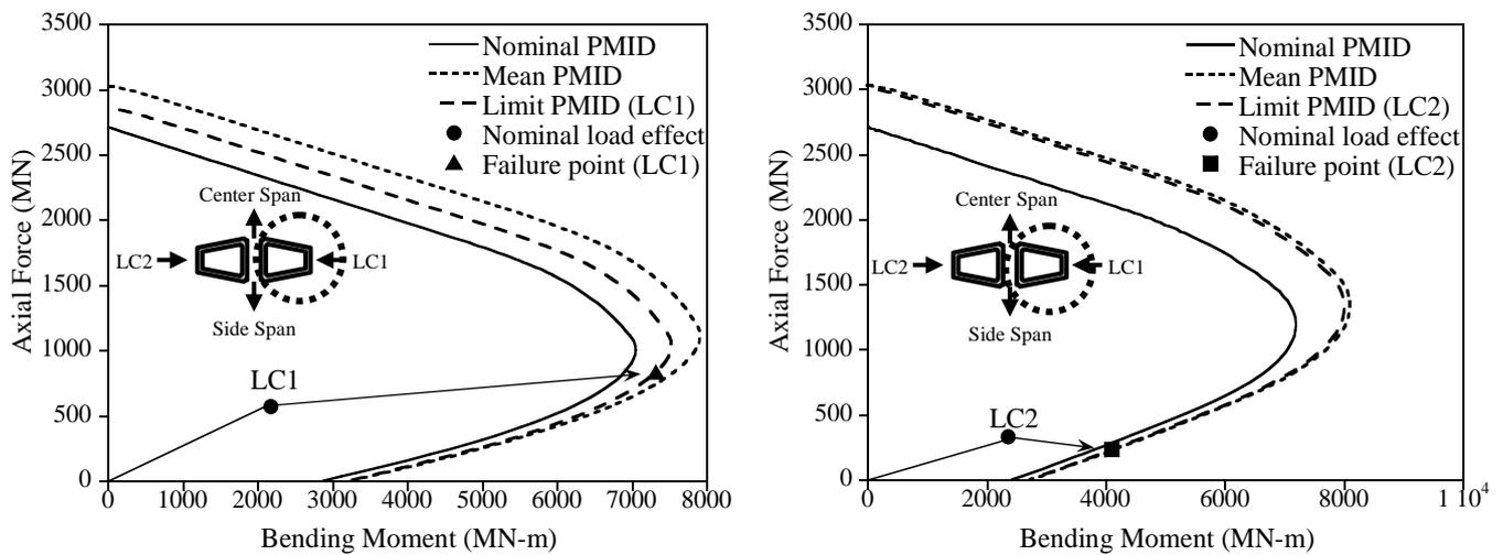
Fig. 1. Failure points and limit PMIDs of transverse wind load
