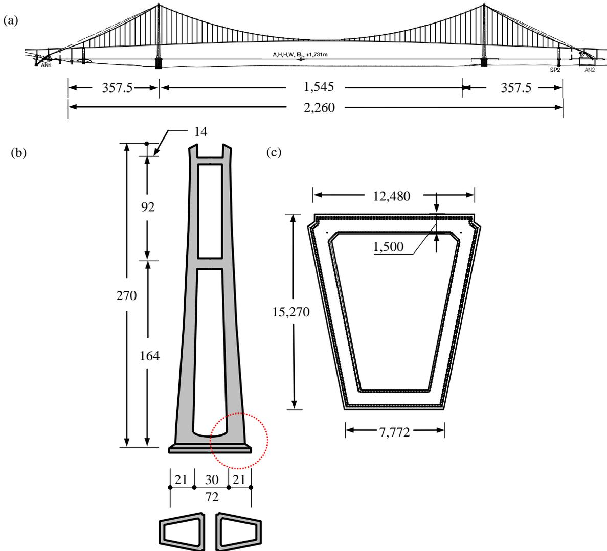
Fig. 1. Yi Sun-sin Bridge: (a) general view (unit: m); and (b) geometry of the pylon (unit: m); and (c) cross section at the bottom of the pylon (unit: mm).
