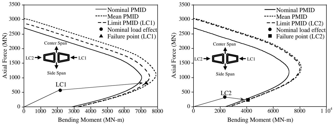
Fig. 2. Failure points and limit PMIDs of transverse wind load
