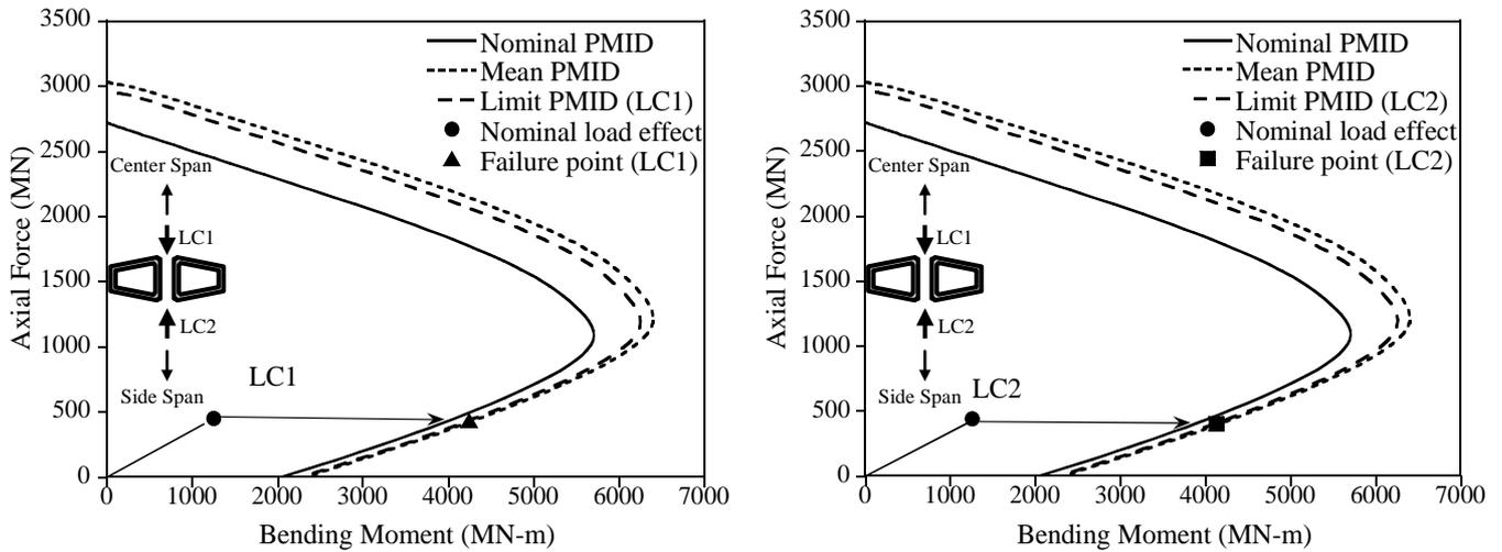
Fig. 3. Failure points and limit PMIDs of longitudinal wind load
