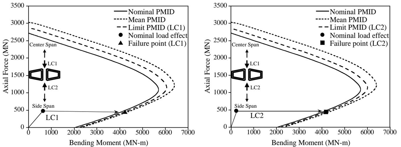
Fig. 4. Failure points and limit PMIDs of service wind load
