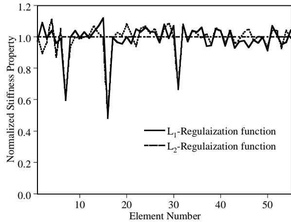
Fig.7 Estimated stiffness properties at the final time step
