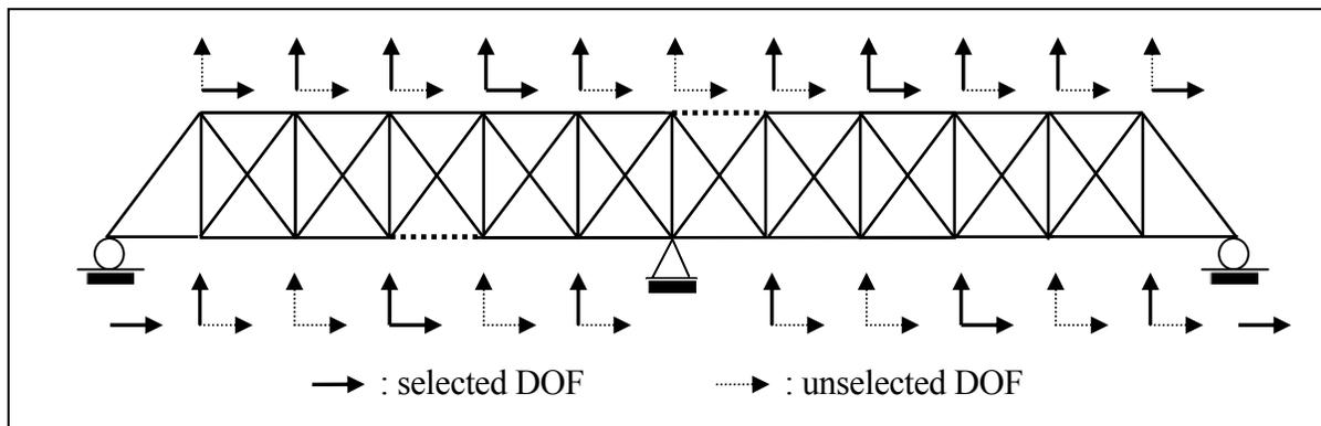
Figure 4. Observation points and directions by optimal sensor placement technique
