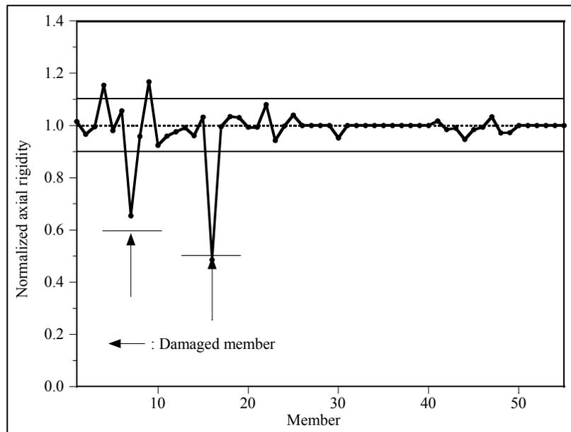
Figure 7. Identified axial rigidities at the final time step
