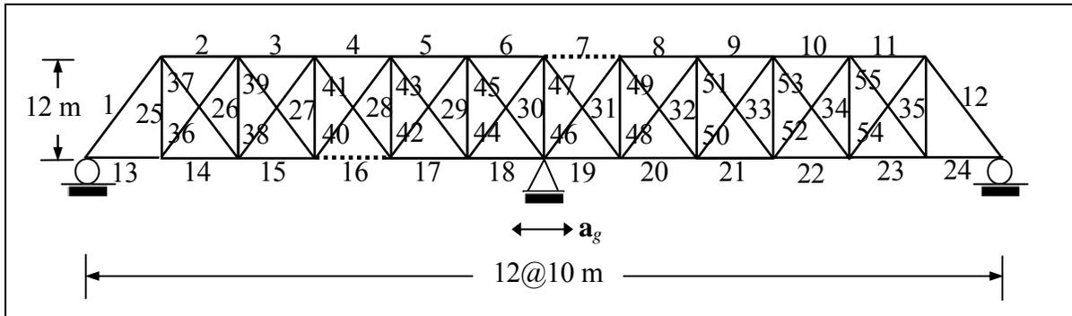
Figure 3. 2-span continuous truss
