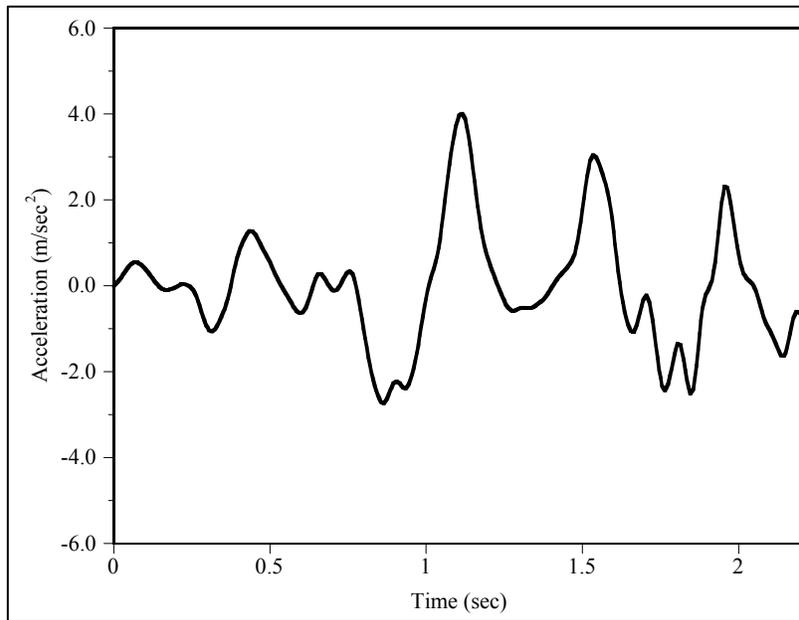
Figure 5. Ground acceleration induced by the Kobe earthquake
