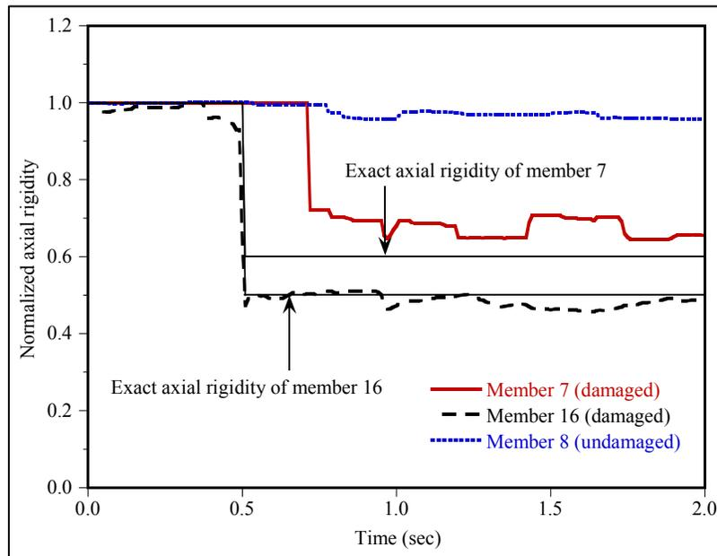
Figure 6. Variation of axial rigidities of two damaged members and one undamaged member
