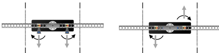
Fig. 2.2. Exciting mechanism of the force controlled forced vibration test
