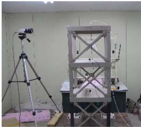
Fig. 4.60 Experimental model 3-story shear building
