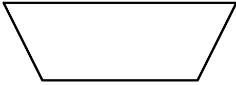
Deformed shape of Bilinear Element for pure bending
