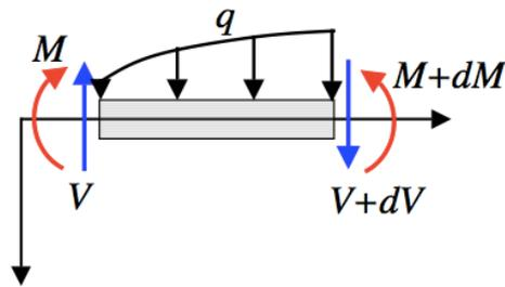
$$\frac{dV}{dx} = -q, \quad \frac{dM}{dx} = V$$
